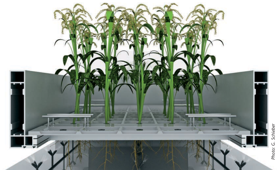
A plant module. An aeroponic cultivation system ensures the supply of water and nutrients.
