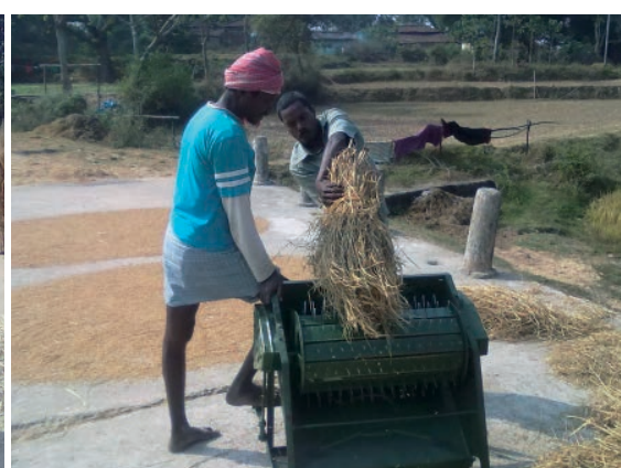
The photo on the left shows traditional methods of paddy threshing which are very labour-intensive and less efficient, whereas on the right, the villagers are using mechanical paddy threshers which are now available at the Common Facility Centers of the project villages.
