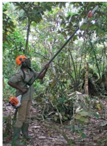
The pole pruner in action in a cocoa plantation. The long extension of the shaft ensures efficient handling and keeps the operator away from the falling biomass.
