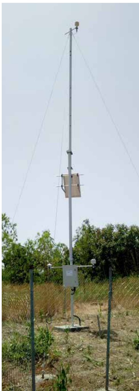
The automatic weather station provides synoptic weather variables such as rainfall, solar radiation, sunshine hours, wind speed and wind direction, air temperature, air pressure, relative humidity and soil temperature at different depths.
