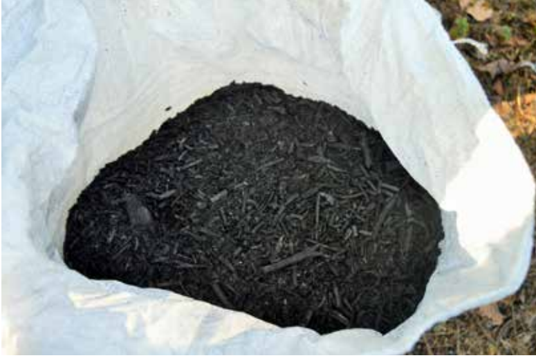
If improved charring kilns are used, the calorific value of the bio-charcoal is about twice as high as with traditional kilns.
