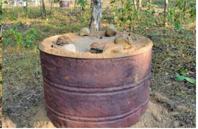
Improved charring kilns allow the controlled burning of the bio-wastes. They are less hazardous in terms of fire and particulate matter.
