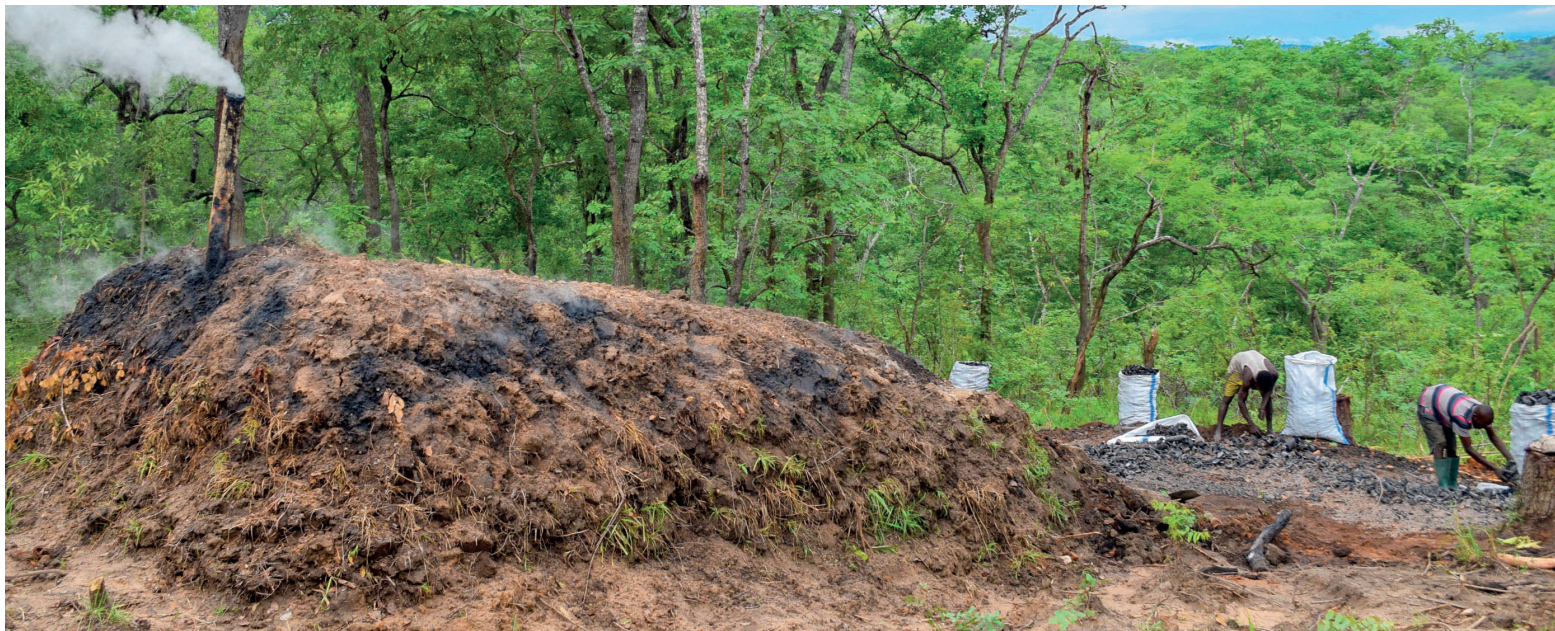
A charcoal kiln in Ulaya Mbuyuni Village using a more efficient kiln structure fitted with a chimney.
