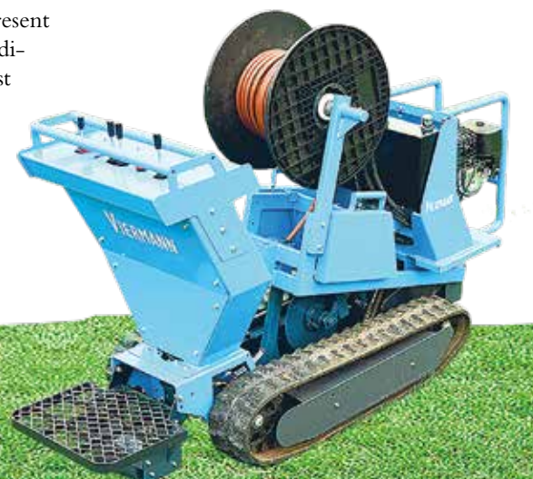
The machine enables pipe installation with minimal disturbance of soil and vegetation.
