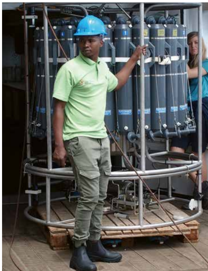
Scientific Production Technician Mbulelo Makhetha with the CTD [Conductivity, Temperature, Depth] rosette aboard the research vessel 'Meteor', during a practical training & research cruise.
