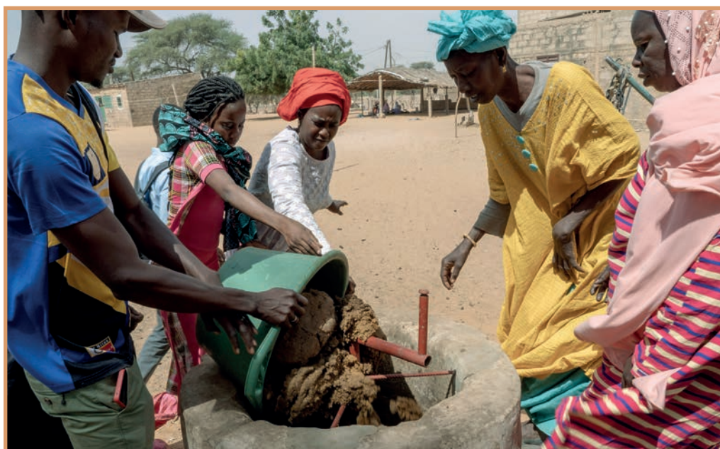
Cow manure is the main substrate used in the biogas plants around Richard Toll.
