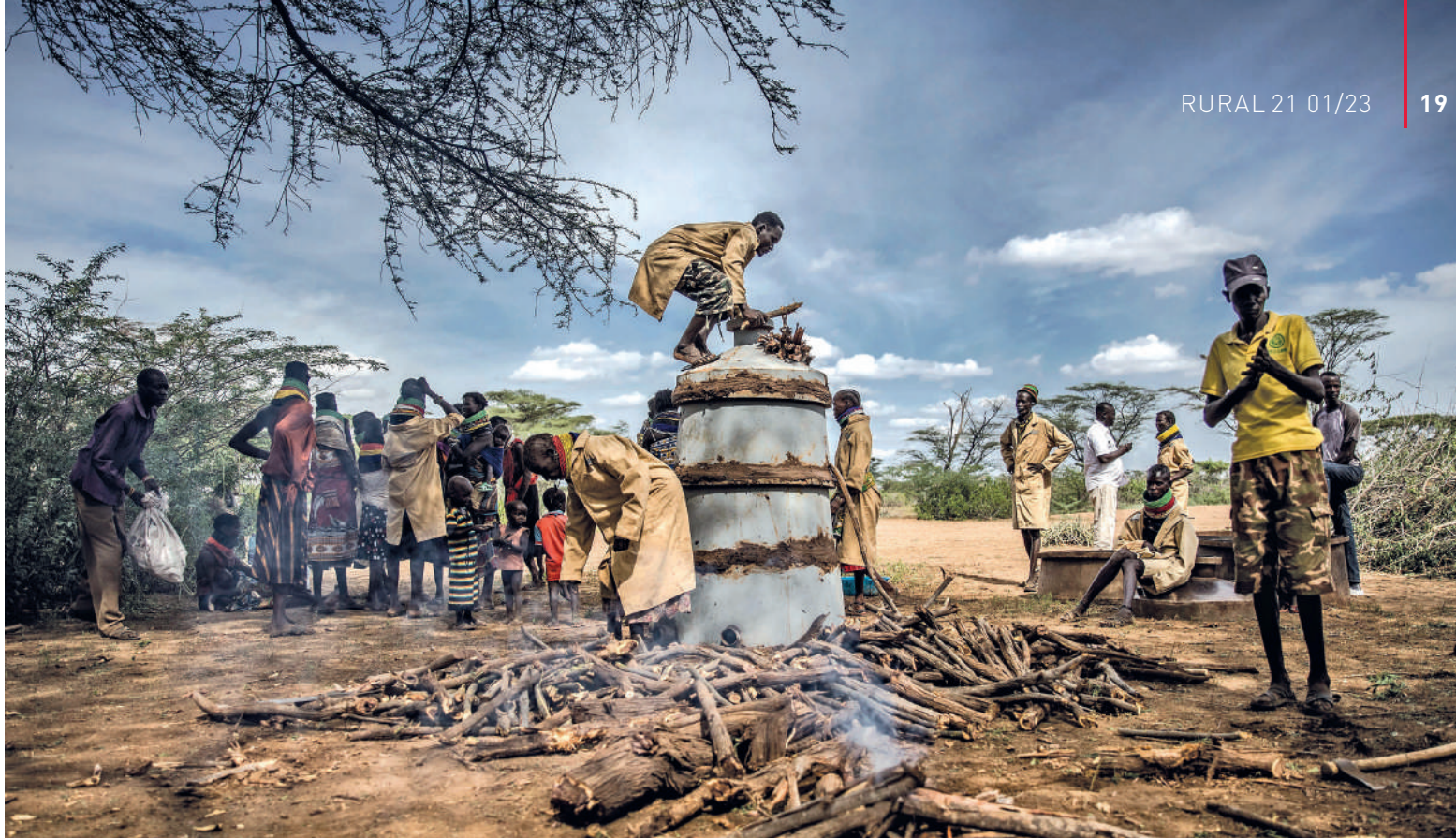
Members of a group belonging to the Turkana community closing a steel ring kiln to prepare charcoal next to their village in Morungole, Turkana County, Kenya. The group has substantially transformed its livelihood, hacking down the invasive trees called Mathenge and turning them into charcoal.
