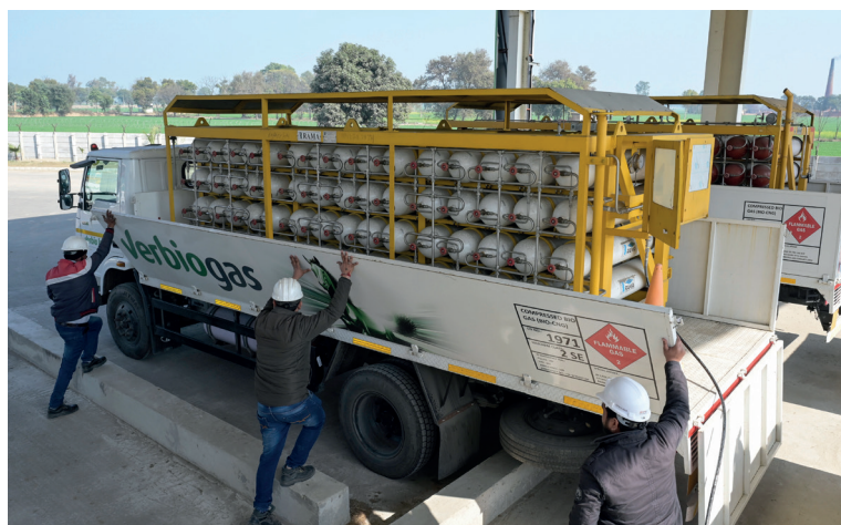
The compressed biogas is filled directly into gas bottles and taken to a petrol station.
